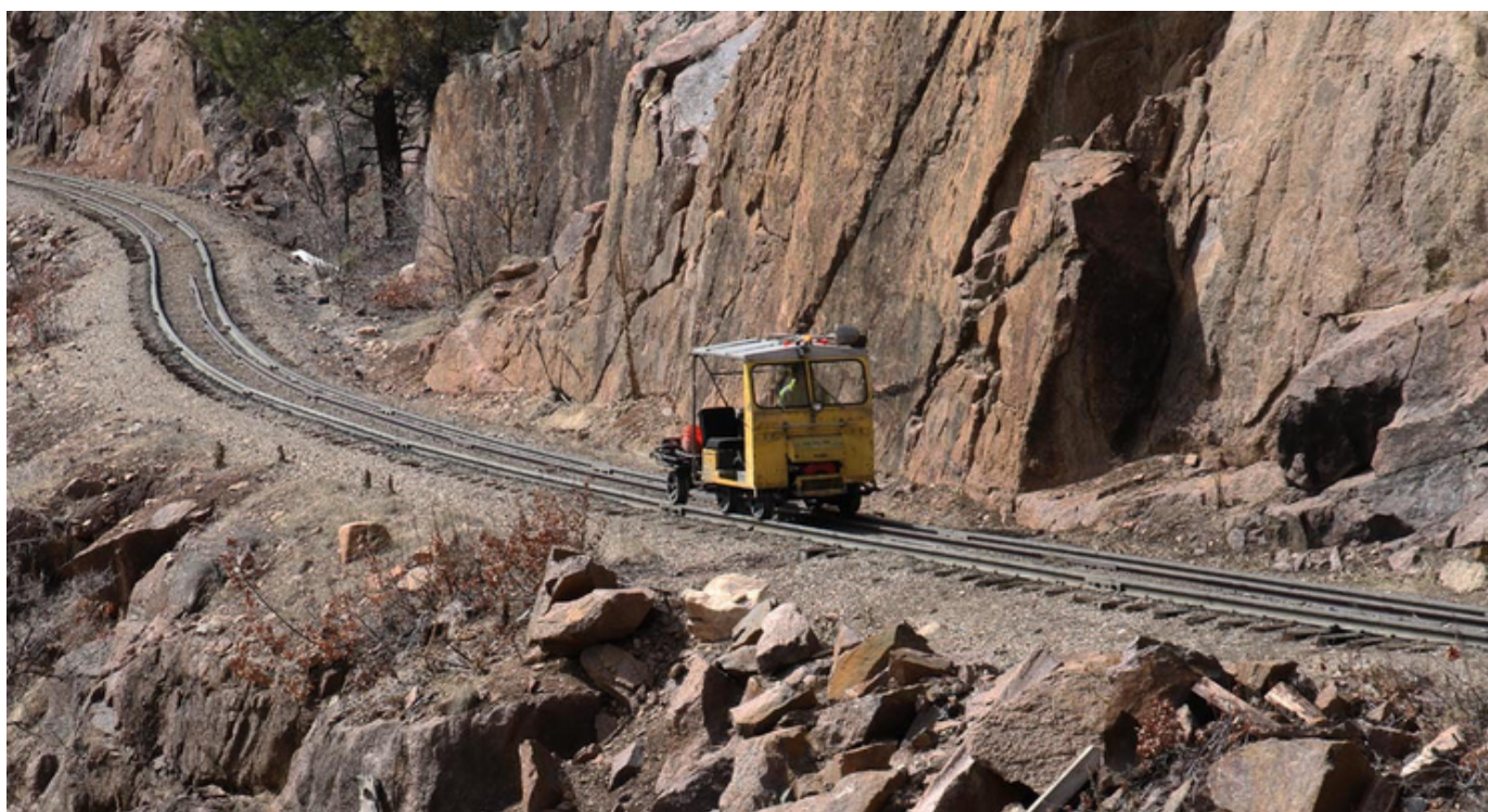
WATCH OUT FOR SPEEDER! – A few minutes after the train to Cascade Wye passed through the canyon, the D&S Fire Brigade speeder appeared. This Fairmont speeder is equipped with a 200-gallon water tank and a long fire hose to knock down any fires the steam locomotive may have started.
